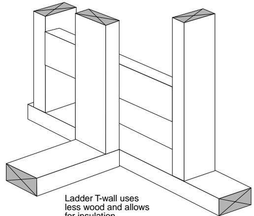
Ladder T-wall uses less wood and allows for insulation coverage behind partition walls
