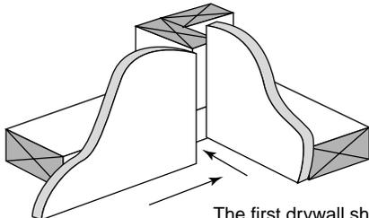
The first drywall sheet is installed against side with clip or backer
